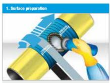
Remove loose coating, smooth out grooves and hollows. Adjacent coating must be completely free of dust, sand and other surface contamination at least 200 mm to the right and left of the damaged area and around the entire circumference. Any contamination that affects adhesion must be removed before application. Roughen the entire coating around the repair area in the peripheral direction with abrasive cloth #40. Then clean the surface.
