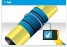
After applying the DENSOLEN® Tape a high-voltage test can be performed according to relevant standards. We recommend the use of spiral or rubber electrodes.
